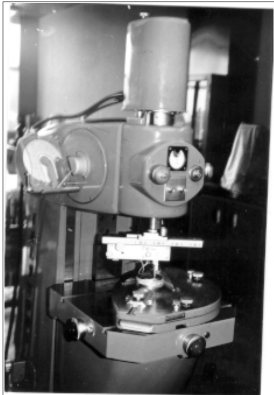
Fig. 7 Set-up used to measure the bearing circumferential wear profile
